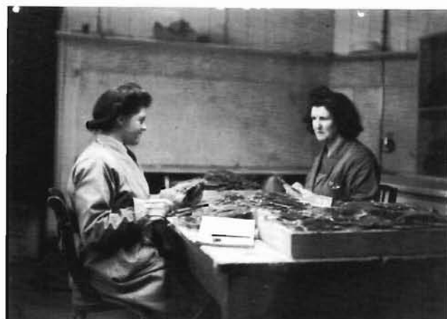
FIGURE 4. Rough splitting of dressed mica books by two workers at the Pitlochry sorting factory. Preparation of mica for the market was a comparatively simple but skilled operation, carried out entirely by hand with the aid of a special splitting knife. Note the heavy gauntlets worn to protect the hands. Any adhering rock was removed before the books were split into plates 3 mm or less in thickness. (BGS Photograph C03808)
