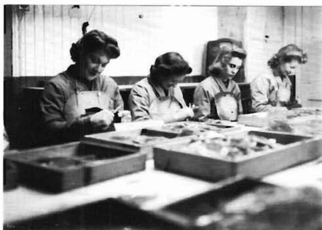
FIGURE 5. Cutting and trimming mica. The split mica sheets were trimmed of all flaws, structural imperfections or, less serious, inclusions. The cutting knife was held at a low angle to the cleavage so the plates were consequently bevelled. (BGS Photograph C03811)
