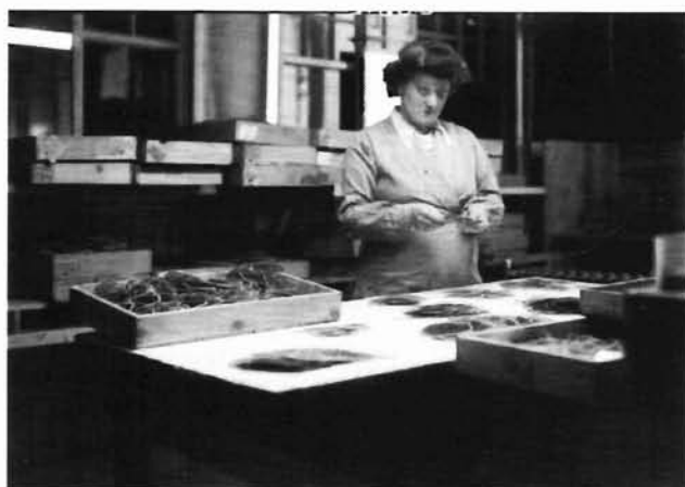
FIGURE 6. Selecting mica sheets for grade and quality. The cut and trimmed mica was sorted into piles of different grade and quality. The grader may also have removed some stained films, etc. to improve the quality. (BGS Photograph C03812)
