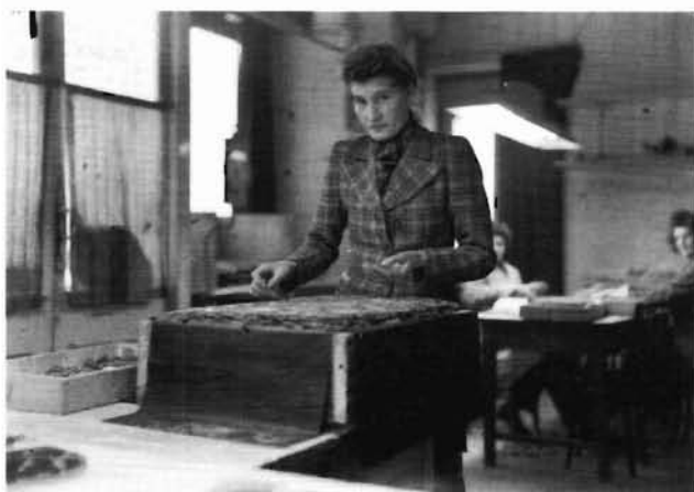
FIGURE 7. Packing graded sheet mica for despatch. Each packing case contained about 50 lb (22–23 kg) of mica, packed in layers with the edges overlapping to prevent damage in transit. (BGS Photograph C03814)
